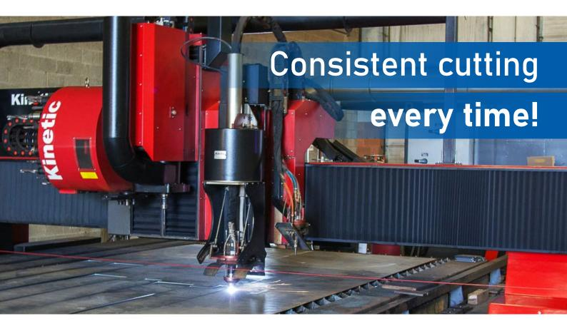
You can count on Rigby Jones to produce excellent results with our HyPerformance Combination Plasma and Drilling system, offering consistent cutting every time in mild steel, Q&T, stainless steel and aluminium. The all-in-one cutting machine can also bevel, tap, countersink and counterbore.
